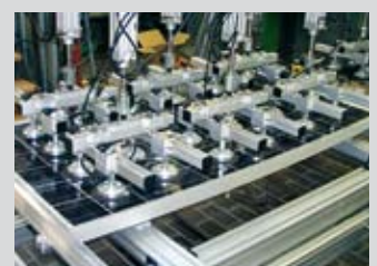
Module load test for AluTec-System©TÜV Rheinland, Germany
